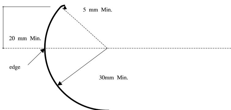
12.5. Recesses in the hull or deck for the purpose of hiding bolt or screw heads etc. are to be permitted. Recesses should be safer than a projecting fixing device in order to be legal. Where recesses are provided to improve safety by eliminating projecting fixing devices, the 5mm radius shall be relaxed as far as it would cover the radius of any transition curve between the deck and the side surfaces of any such recess.
